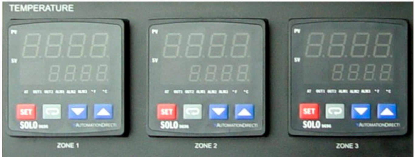
Figure 1-15 Zone Temperature Controllers
