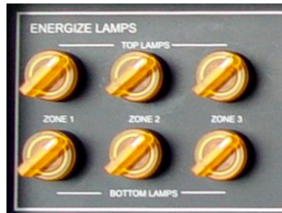
Figure 1-14 Energize Lamps Controls
