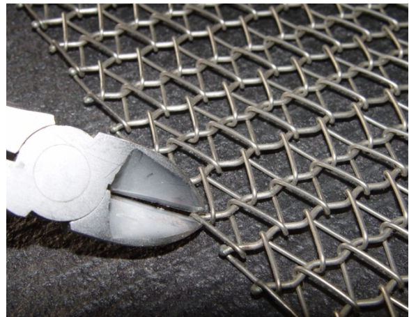
Figure 2.1 Cut Wire at Ball Joint
