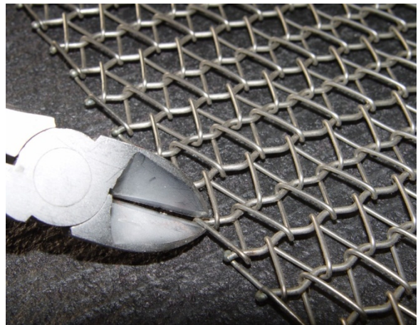
Figure 2.1 Cut Wire at Ball Joint
