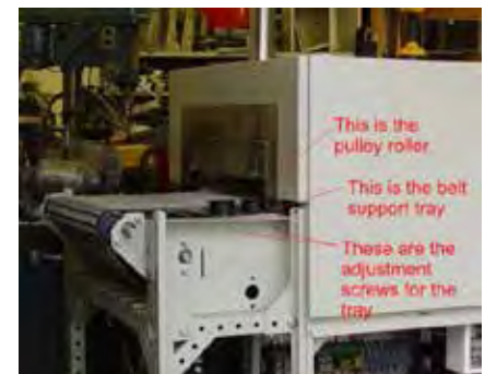
Adjustment screw location (furnace exit)
