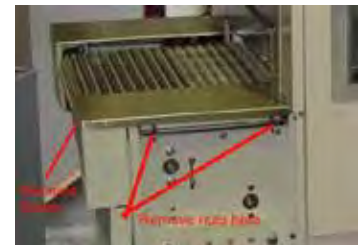
Top covers at furnace exit
