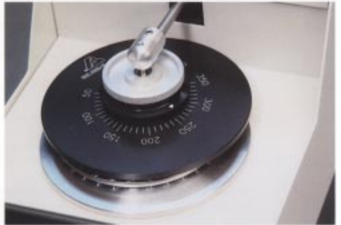
Precision Thinning Attachment enables SEM and TEM samples to be prepared.
