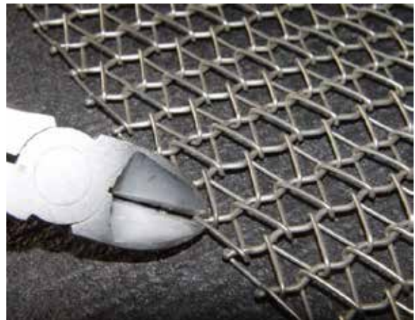
Figure 2.1 Cut Wire at Ball Joint
