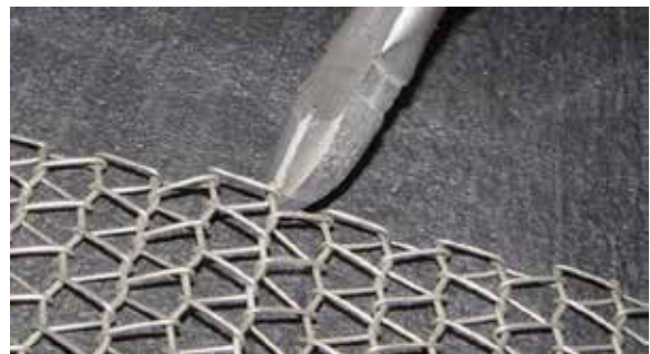
Figure 2.2 Second Cut at Opposite Side
