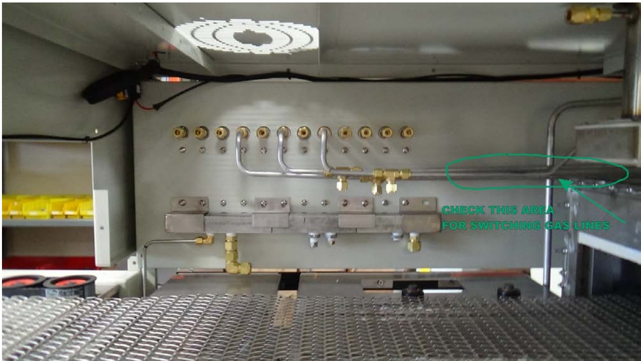
Figure 6-5. ALTERNATE PLACE TO SWITCH LINES
