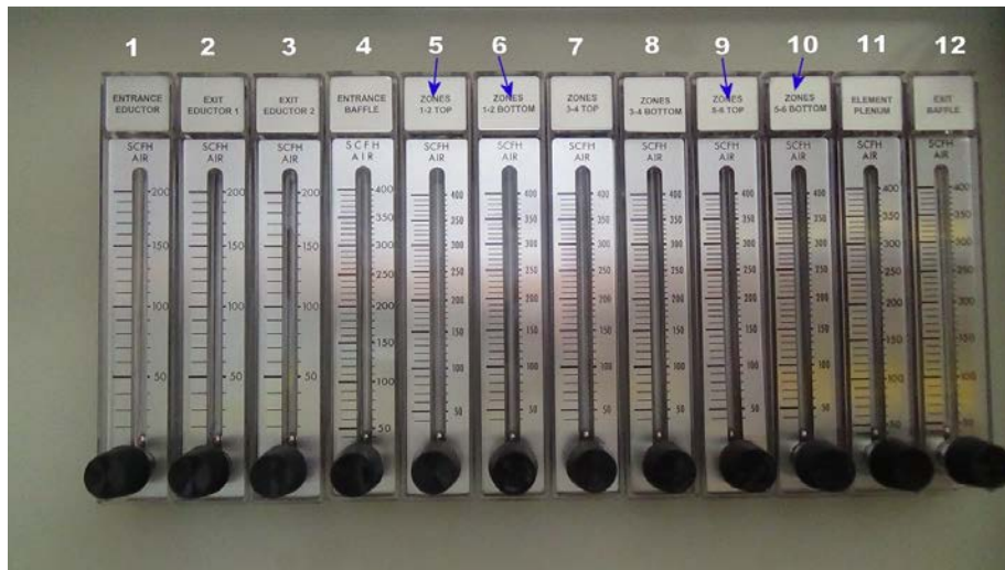
Figure 6-1. FLOWMETER PANEL REFERENCE
