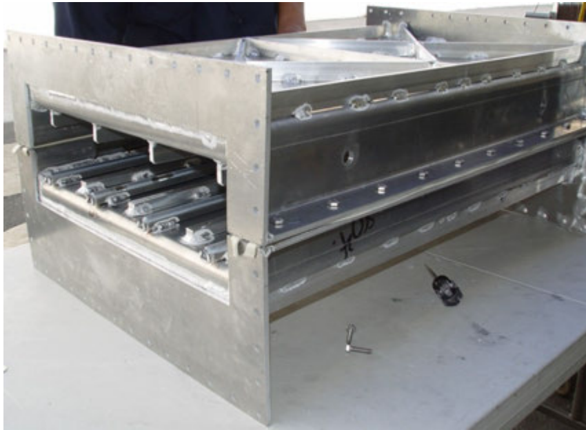
New Cooling Section with quartz rods
