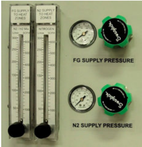
Figure 2-14 Supply Gas Mixing System
