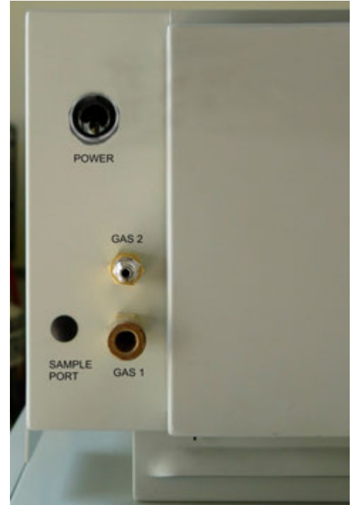
Figure 2-12 Process Gas Connections
