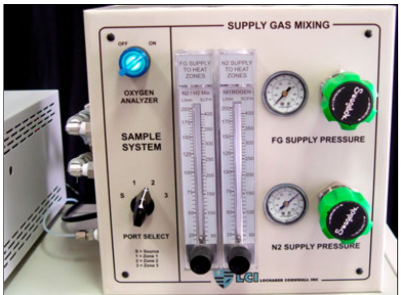
Figure 3. Turn Sample System ON and select Port
