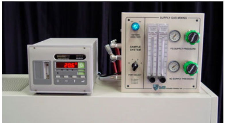
Figure 1. Position oxygen analyzer on furnace
