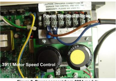
Figure 2 Power connect from 3984 module
