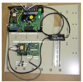
Figure 1 Motor control Panel Layout
