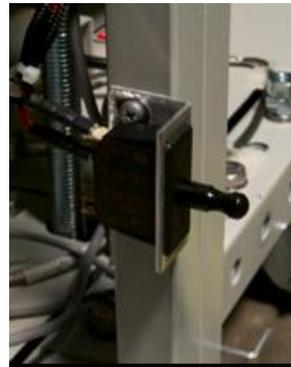
Panel Switch Installed - Bypass Mode Position
