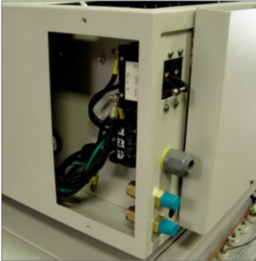
Figure 6-5 Control Console showing 3 options: Circuit Breaker; Dual Process Gas; & Sample Port
