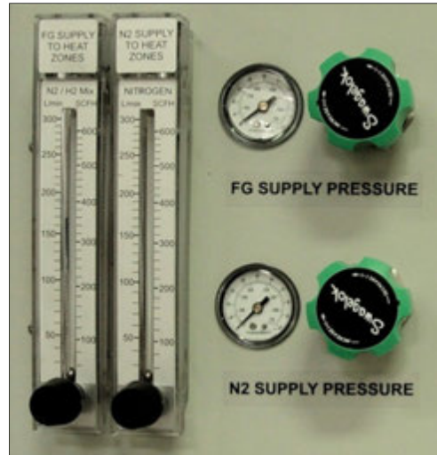
Figure 6-6 Controls for Supply Gas Mixing System. (Only available on Dual Gas Furnaces)
