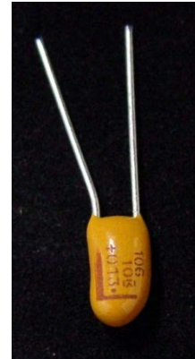
Typical tantalum capacitor showing polarity, positive (+) is on left
