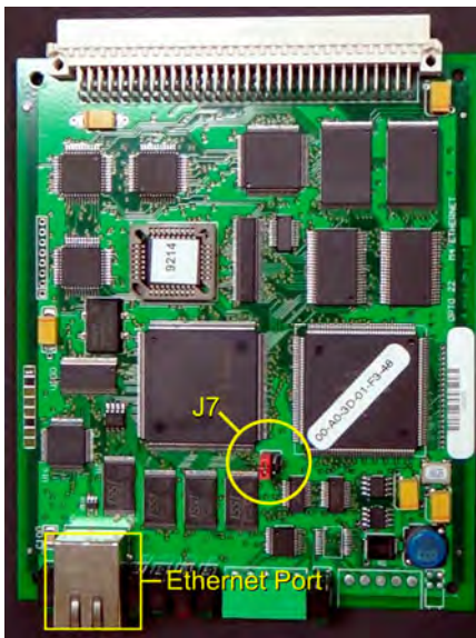
Figure 3-29 Location of J7 Jumper J7 in Normal RUN Position
