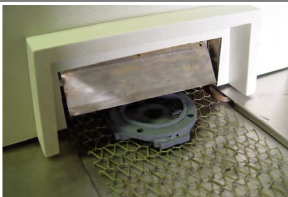
Figure 8-11 Brass forging sample exiting furnace
