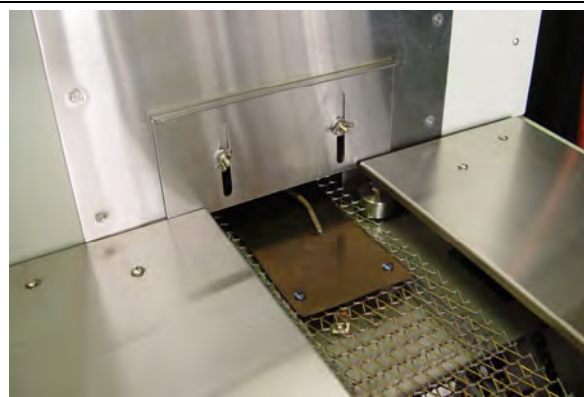
Figure 8-12 Sample plate exiting furnace
