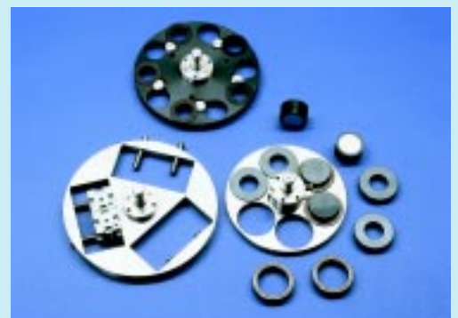
A complete series of specimen holders accommodates both compression and cold mounted samples as well as a broad range of large unmounted and irregularly shaped specimens.
