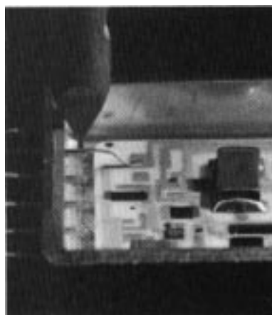
A Unitip electrode used to bond gold ribbon to hybrid inter-connect pin.
