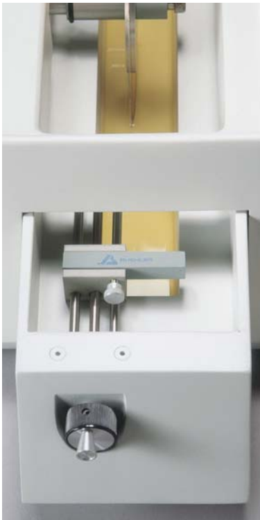
Dressing chuck is conveniently located within the coolant tray.
